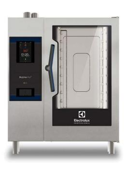
219609 (ECOE101K3I30) SkyLine ProS Combi Boilerless Oven with touch screen control, 10x1/1GN, electric, 2 cooking modes (recipe program, manual), automatic cleaning, spray gun, 6-sensor probe, 3-glass door and IoT module - 480V US
